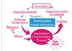
In our laboratory, solid / solid separation and concentration technology without heating / dissolving the waste or refractory ore is studied to achieve an energy-saving separation and concentration process. This process is regarded as "pre-treatment" or "middle treatment" before metallurgical / hydrometallurgical process, which produces high-purity metal.
