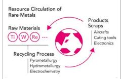
Our laboratory is developing new, efficient and environmentally sound processes to recycle rare metals for which an increase in demand is expected, such as titanium, tungsten, cobalt, rhenium and platinum group metals.
