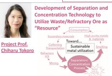
Tokoro Laboratory explores solid—solid separation and concentration technology without heating or dissolving the waste or refractory ore to achieve an energy-efficient process. This process is considered "pretreatment" or "middle treatment" performed before the metallurgical/hydrometallurgical process that produces high-purity metals.
